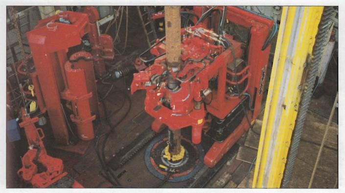
In response to Norwegian Petroleum Directorate regulations limiting personnel on the rig floor, Weatherford Norway has developed a casing modem with remote-controlled power tongs.
