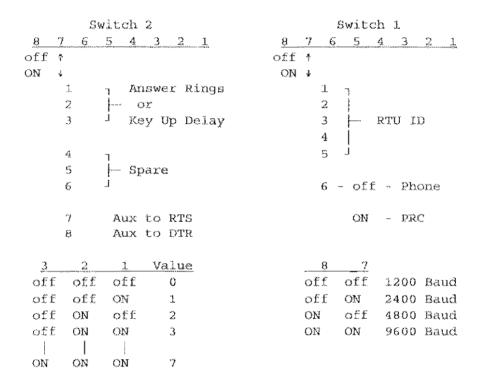
Rings, Key Up Delay, and RTU ID are set as binary numbers.
