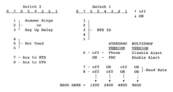
The RTU ID and Key Up Delay are set in binary as shown below:
