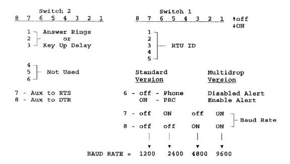
The RTU ID and Key Up Delay are set in binary as shown below:
